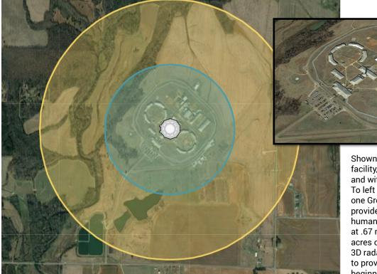
Shown is a US-based correctional facility, covering 1,600 acres and with 2,100-inmate capacity. To left is an illustration of how one GroundAware radar system provides automated detection of humans at .31 mile and vehicles at .67 mile -- that's more than 300 acres covered with one sensor. 3D radar options are available to provide coverage of drones, beginning at nearly 1 mile.
